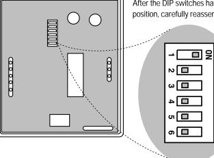
After the DIP switches have been set to the desired position, carefully reassemble the thermostat.
